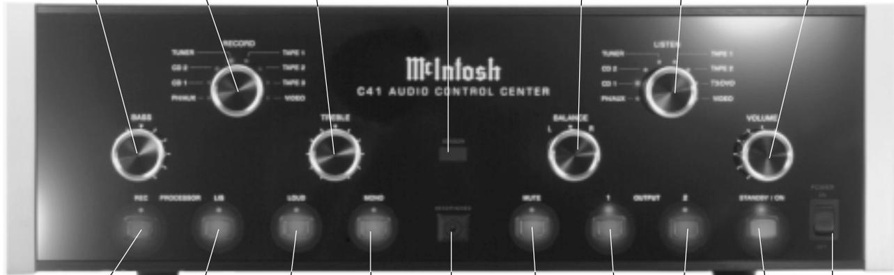
REC PROCESSOR push-button turns the Record Processor loop on or off
