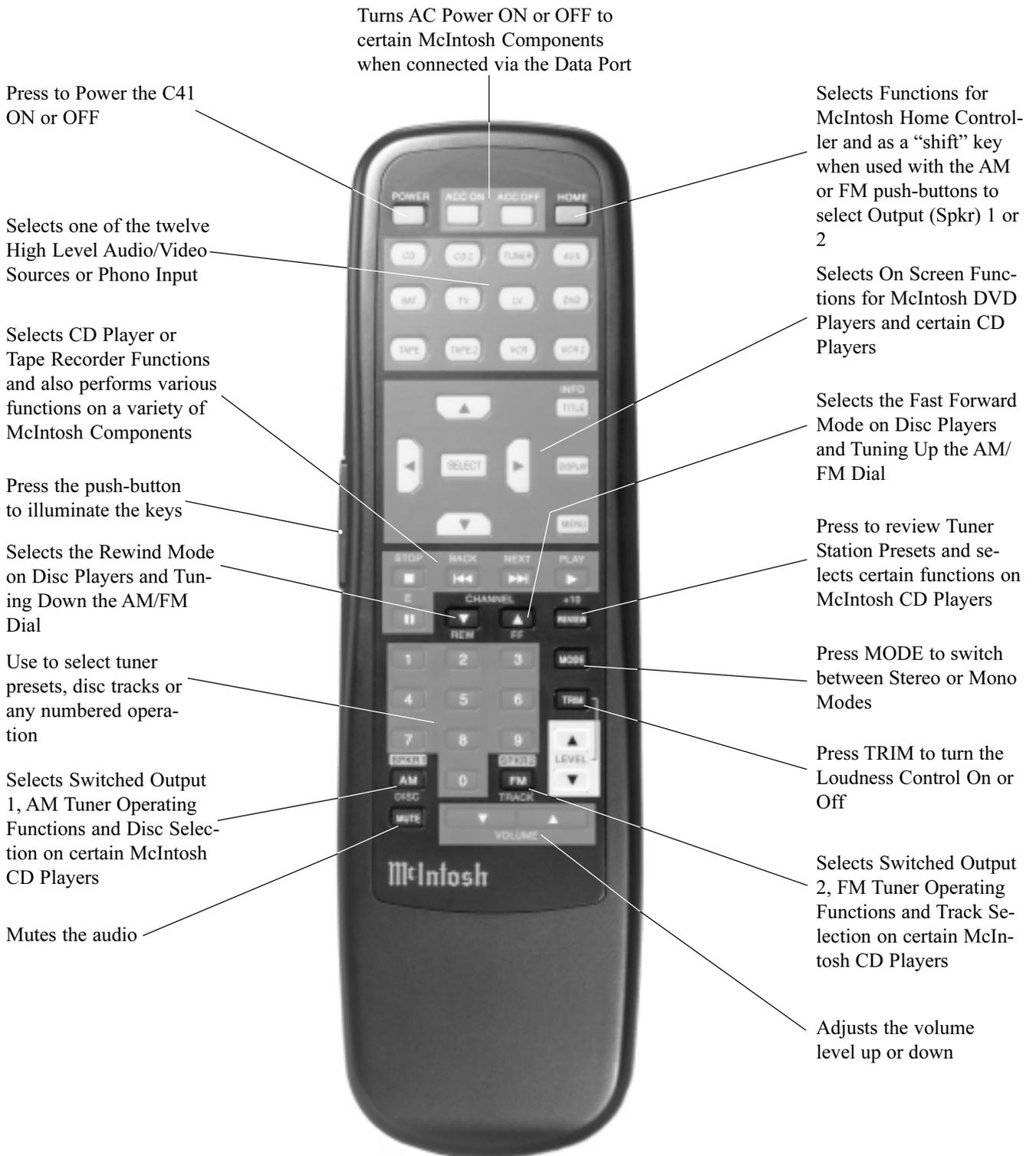
*Note: The Remote Control push buttons that are highlighted in white are for use with other McIntosh Control Centers.*
